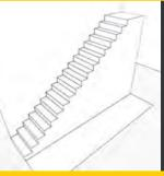
A typical straight staircase leads up to the next floor without any middle landings.
