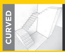
A curved staircase has a straight set of steps leading to a landing and then additional steps leading onto the next floor.
